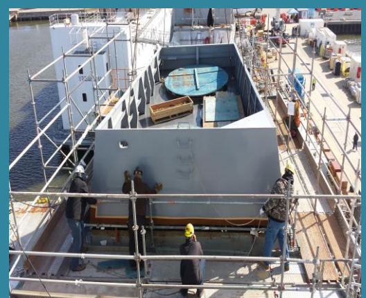
Painted New Stack being put into place
